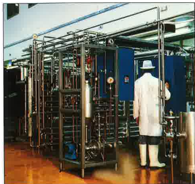
Steritube Pilot Plant installed at the premises of the Leatherhead Food Research Association, UK.
